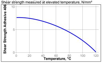
Grit Blasted Mild Steel to Polypropylene Shear strength measured at elevated temperature, N/mm<sup>2</sup>
